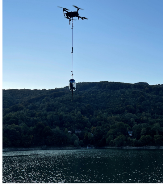
Fig. 6.2 UAV-based measurement platform, Lopy modules and Pytrack expansion board for GPS coordinate monitoring
