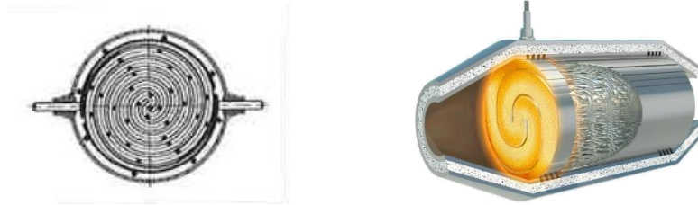
Figure 6 Emitec EHC build cross-section [3.2] and cut-out [3.1]
