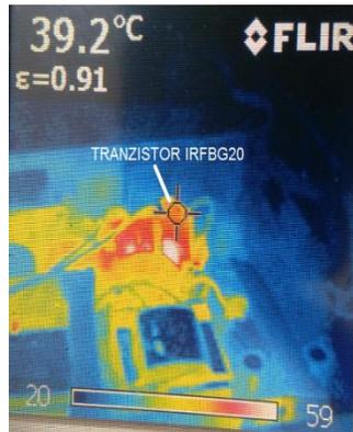
Figure 4.26. Temperature value of transistor with reduced cooling fan speeds [78]
